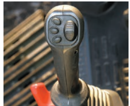
Joysticks with proportional control button for attachments are standard
